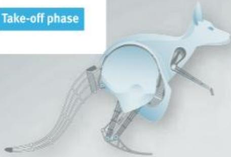
1 Pretensioning the elastic spring element
